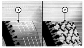
1 — Worn Tire 2 — New Tire These indicators are molded into the bottom of the tread grooves. They will appear as bands when the tread depth becomes 1/16 in (2 mm). When the tread is worn to the tread wear indicators, the tire should be replaced.
